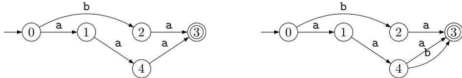
**Figure 3.** Automata  $\mathcal{B}_X^1$  (left) and  $\mathcal{A}_X^2$  (right) for  $X = (aaa, ba, aab)$ . The automaton  $\mathcal{B}_X^1$  is equivalent to  $\mathcal{A}_X^1$  and it is obtained from  $\mathcal{A}_X^1$  by doing a copy of the path from 0 to 4 with label  $aa$ . The automaton  $\mathcal{A}_X^2$  is obtained by adding the edge  $(4, b, 3)$
