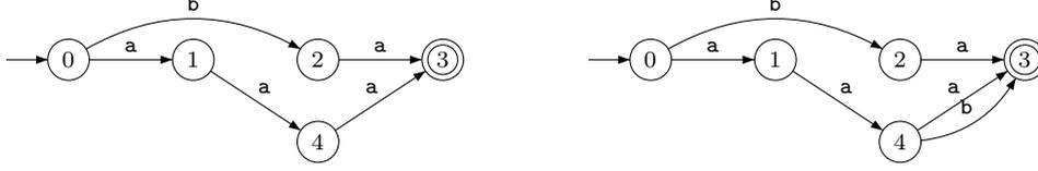
Fig. 3. Automata  $\mathcal{B}_X^1$  (left) and  $\mathcal{A}_X^2$  (right) for  $X = (\text{aaa}, \text{ba}, \text{aab})$ . The automaton  $\mathcal{B}_X^1$  is equivalent to  $\mathcal{A}_X^1$  and it is obtained from  $\mathcal{A}_X^1$  by doing a copy of the path from 0 to 4 with label  $\text{aa}$ . The automaton  $\mathcal{A}_X^2$  is obtained by adding the edge  $(4, \text{b}, 3)$
